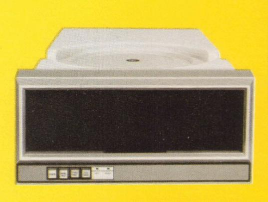
Precision control over tape speeds of 25 to 45 ips comes from an optical tachometer and fully controlled dynamic braking. Encodercontrolled speed assures both short and long-term stability.
